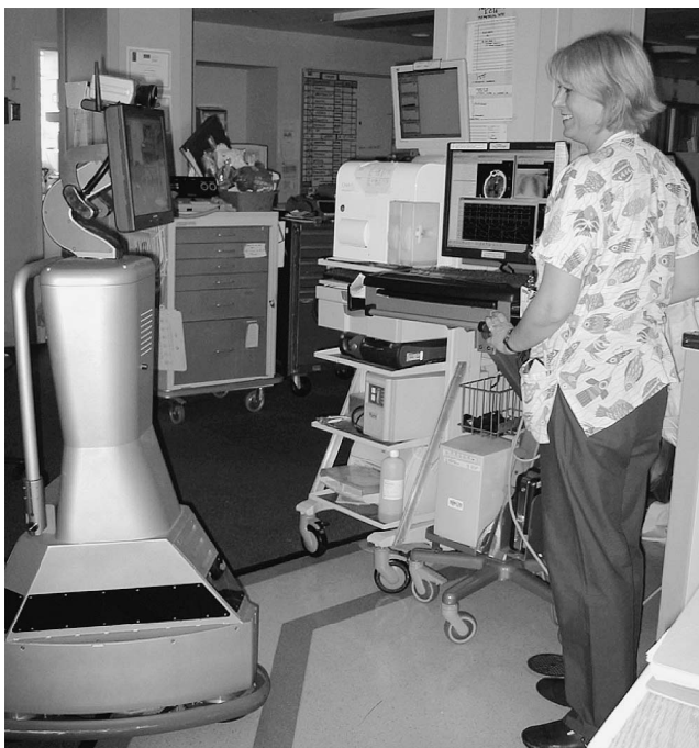
Figure 3. The telepresence robot is shown in our intensive care unit interacting with the bedside nurse
