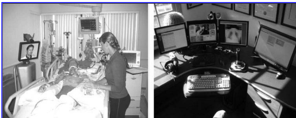
Fig. 2. Left image above showing a robot that has arrived at the bedside of an ICU patient. The clinician is then able to visually examine the patient, review all graphics and function of life support devices, and converse directly with the bedside nurse. Right image: MD Home Tele-ICU indicating the Clinical Information System on left-hand monitor, the view through the robot in the middle monitor, and the radiographic images on the right screen. On an independent screen to the far right is a clinical knowledge base (Up-to-Date, Wortham, MA).
