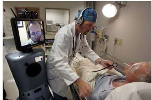
From his office at Sutter Medical Center, Dr. James Finn, the medical director of Healdsburg District Hospital's intensive care unit, directs registered nurse Mark Blankenship as they listen to the heart of patient John Reininga. The hospital's new Remote Presence Robotic System will allow specialists to examine rural patients from anywhere in the world using a laptop and a joystick. Photo by John Burgess/The Press Democrat (Photo by - John Burgess)
