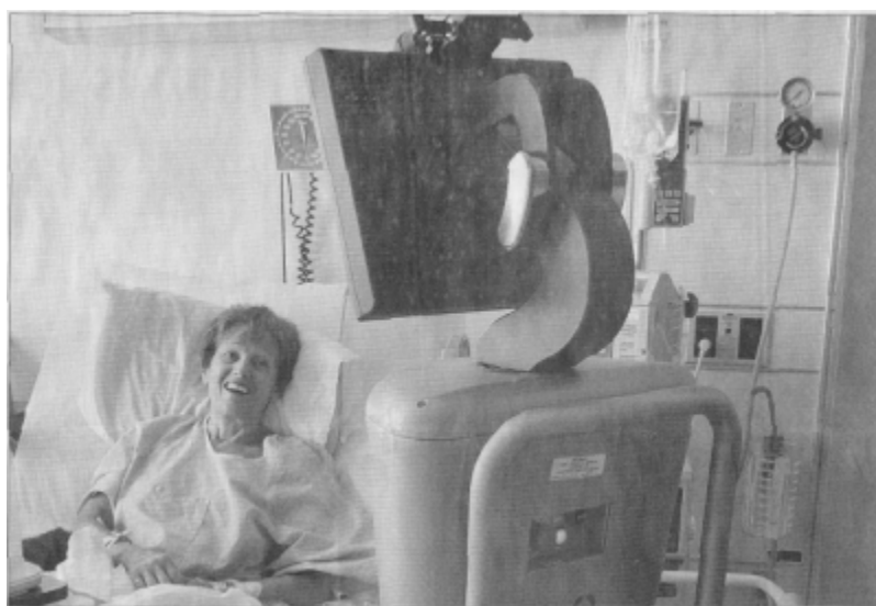
Doctor and patient converse via microphone in the videocamera and speaker in the robot's midsection. Doctor can use videocamera to take pictures of patient or patient's surgical area for analysis.
