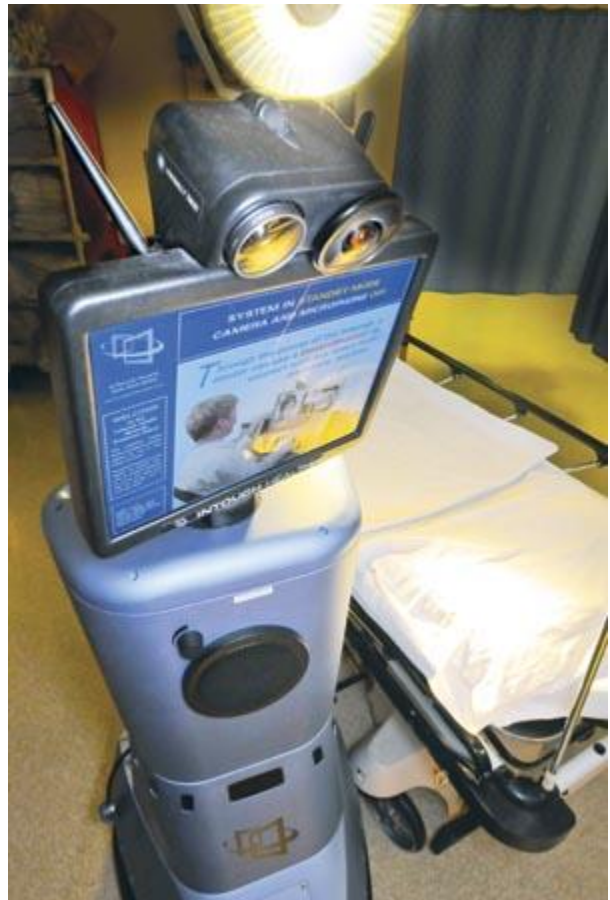
The Remote Presence Robot, or RP-7, above, will be stationed on permanent call at Lompoc Valley Medical Center to help in the emergency diagnosis of the worst stroke cases when the neurologist is not in the hospital.//Len Wood/Staff
