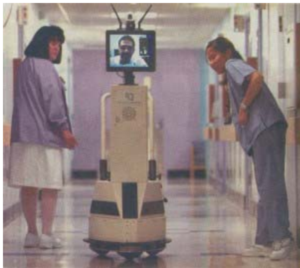
R2-D2 WITH AN M.D.: Operated by remote control, a robot can allow patients to have a virtual visit with their doctor when the doctor cannot be physically present.
